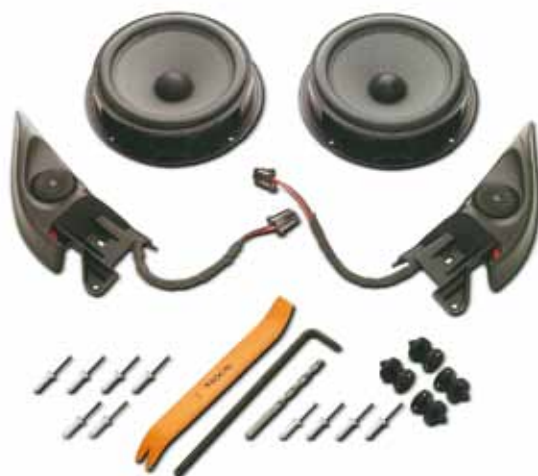
IFVW Golf 6: 2-way component kit, user manual, video and specific tools for mounting. Compatible tweeter mounting, integrable and with harmonious design.
